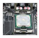
11. Visually inspect if the CPU is seated well into the socket, then remove the CPU Clip with 2 fingers. Then cover the load plate onto the package.
